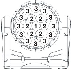
Pixel Zone Layout 44 Ch. Mode (45 Ch. Mode w/ Software Version <u>></u>6.1)
